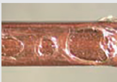
● 表面涂层脱落 Surface coating peeling
